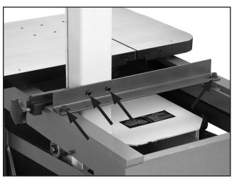
Figure 8. Removing shipping bracket.
